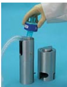
STEP 1: Insert Venti-Scan™ IV Kit in canister
